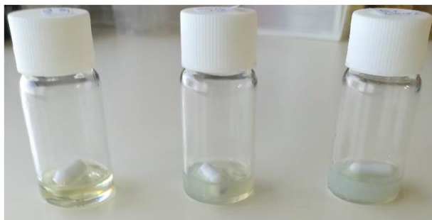
Fig. S5 PET in thymol:carvacrol (1:1) samples at room temperature, after full PET solubilization at 150°C. PET/ES ratio from left to right 1:10, 2:10, 3:10.
