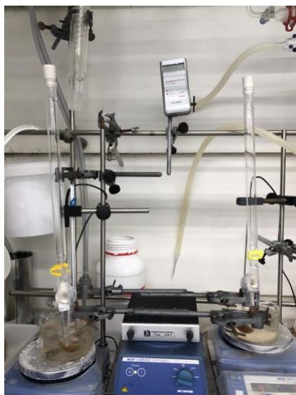
Figure S1. Set up used for the heterogeneous Mitsunobu coupling reaction
