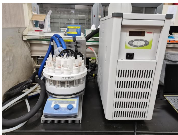
Fig. S12 Photocatalytic sugar-to-LA conversion setup.
