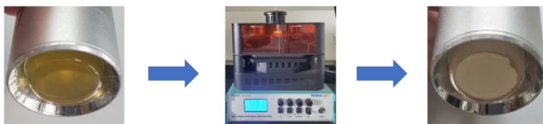
Before the reaction Photocatalytic reactor After the reaction Figure S16. The images showing the photocatalytic oxidation of p-xylene into terephthalic acid. The white precipitate can be observed after the reaction.
