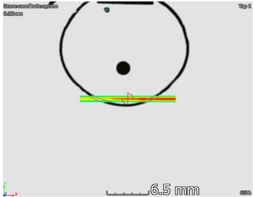
Figure 31. The 2D intensity map of the neutron beam as it passes through the object in measurement position 3 (from right to left, cut at the centre plane of the neutron beam)
