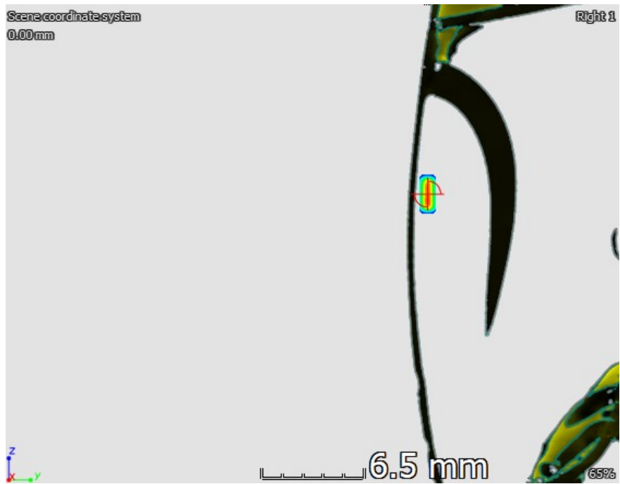
Figure 32. The 2D intensity map of the neutron beam as it passes through the object in measurement position 4 (beam's eye view, cut at the centre of the object)
