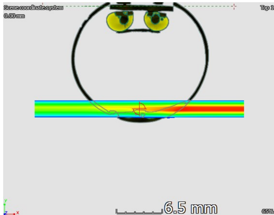
Figure 14. The 2D intensity map of the neutron beam as it passes through the object in measurement position 2 (from right to left, cut at the centre plane of the neutron beam)
