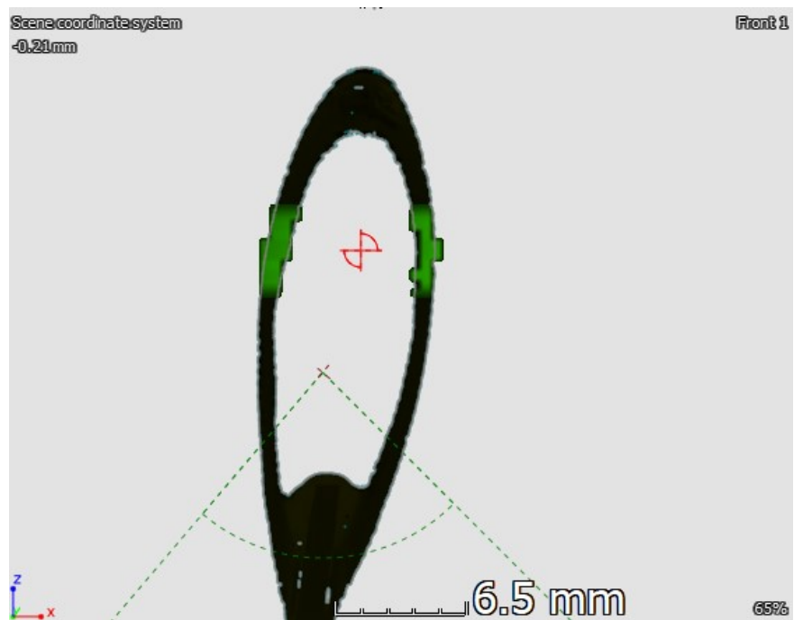
Figure 34. The 2D emission intensity map of element Fe (cut at -0.2 mm relative to the centre of the neutron beam)
