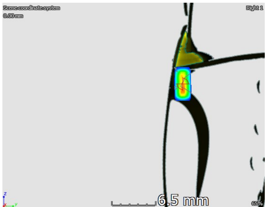
Figure 16. The 2D intensity map of the neutron beam as it passes through the object in measurement position 2 (beam's eye view, cut at the centre of the object)
