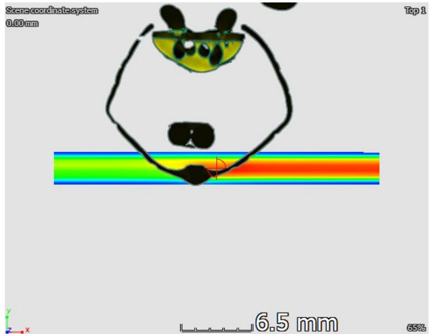
Figure 39. The 2D intensity map of the neutron beam as it passes through the object in measurement position 4 (from right to left, cut at the centre plane of the neutron beam)
