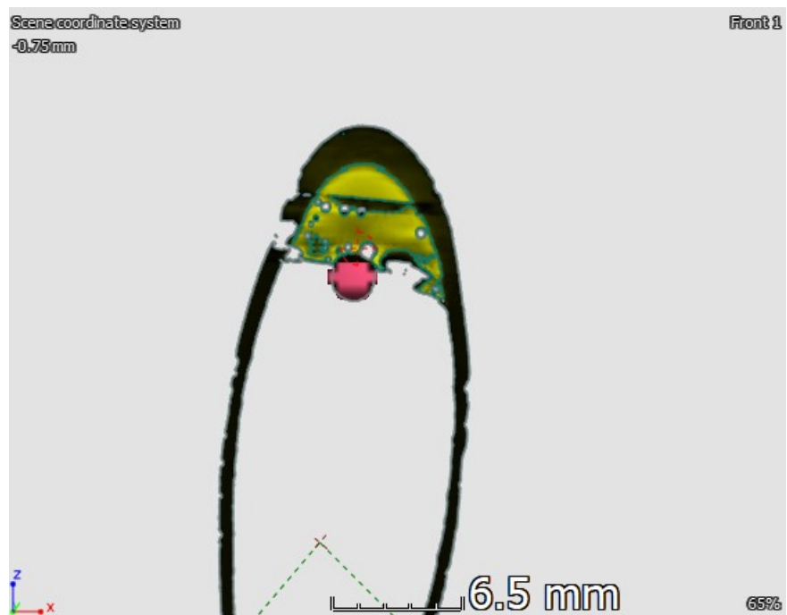
Figure 28. The 2D emission intensity map of element Zn (cut at -0.8 mm relative to the centre of the neutron beam)
