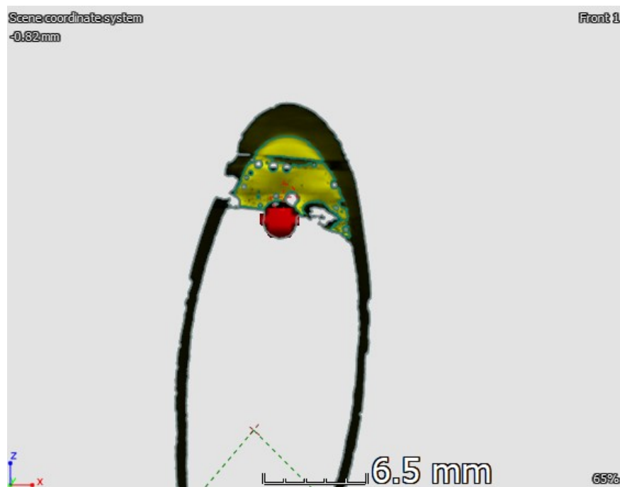
Figure 26. The 2D emission intensity map of element Cu (cut at -0.8 mm relative to the centre of the neutron beam)
