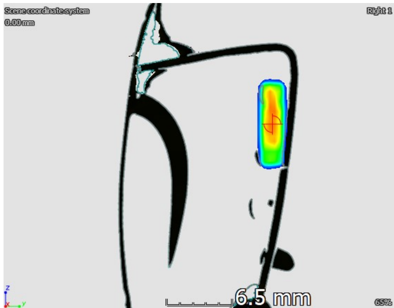
Figure 4. The 2D intensity map of the neutron beam as it passes through the object in measurement position 1 (beam's eye view, cut at the centre of the object)
