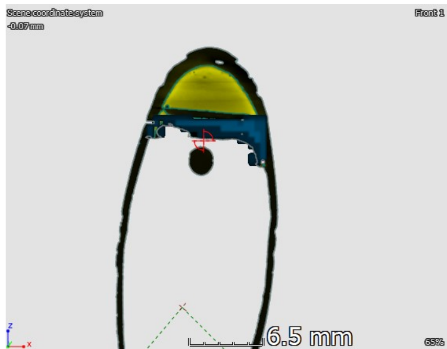
Figure 22. The 2D emission intensity map of element Pb (cut at the centre of the neutron beam)
