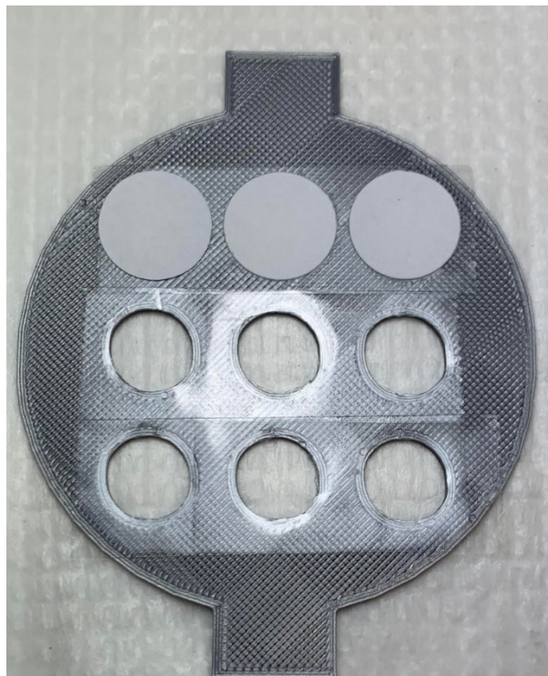
Figure S6. Image of the 3D-printed ELISA plate that was used to secure each 16mm-diameter filter cutout (top row) containing different concentrations of antigen. The holes in the array are 12mm in diameter and double-sided tape was placed over each row prior to cutting out the interior with a blade.
