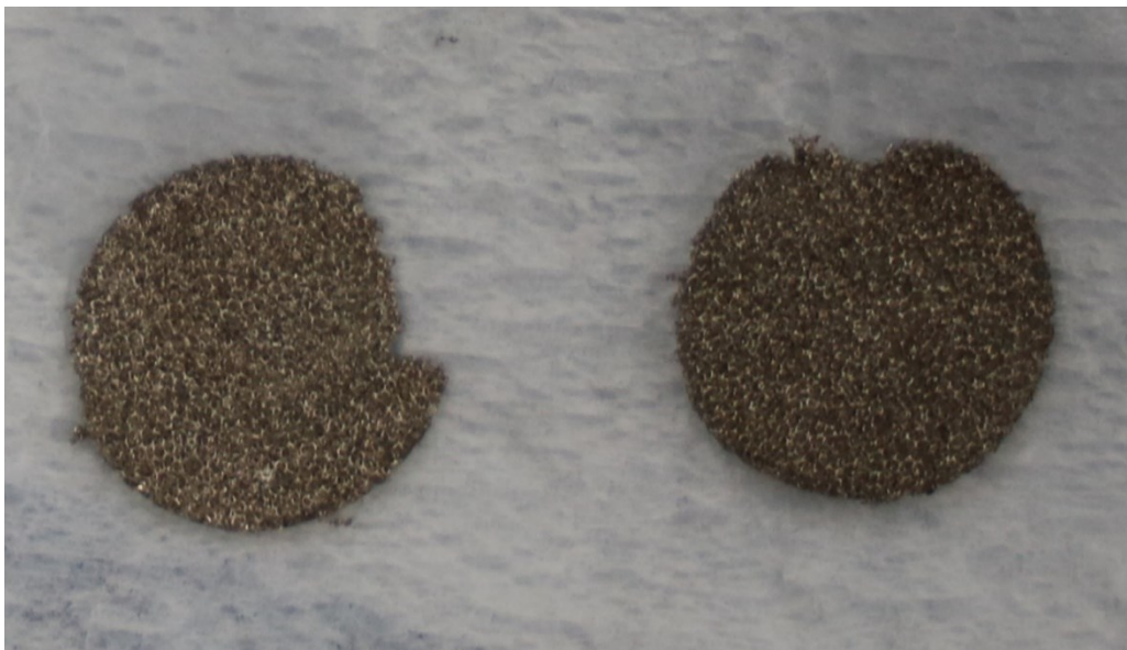
Figure S11. Photographs of dismantled symmetric cells which are molten Li surface coated on Ni-foam. The foam surface coated with molten Li became brittle after coin cell fabrication, which resulted in a short circuit.
