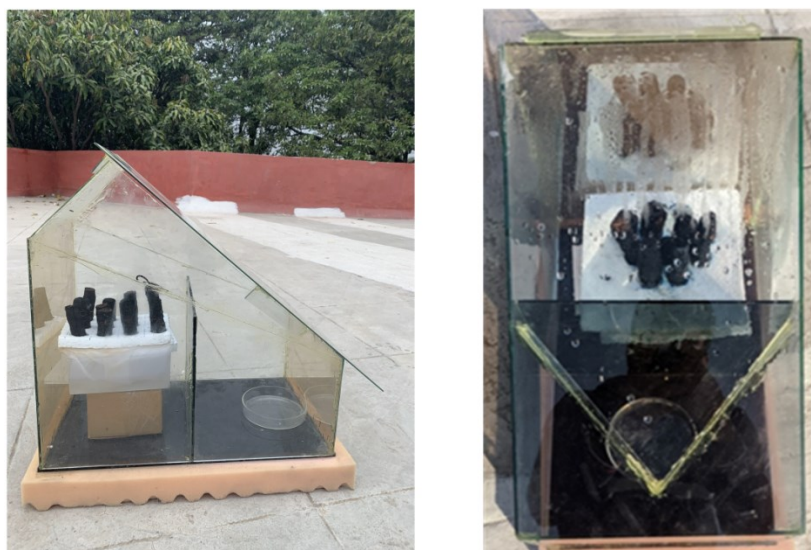
Fig. S7. Photograph for the side view (left) and top view (right) of the prototype of CCH based solar steam generation.
