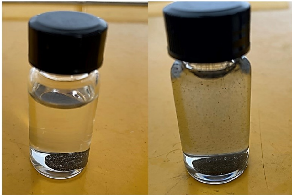
Figure S8 Immersion experiment in ultrasonic environment. (a) NCS on the surface of NiCu alloy. (b) NCS on the surface of Ni foam.
