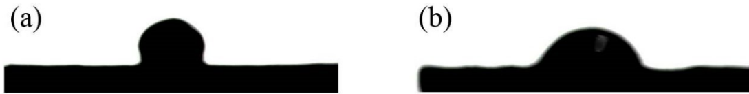
Fig. S7 Contact angle of LM and BN films. (a) LM was dropped on the BN film directly. (b) LM was rubbed on the BN film.
