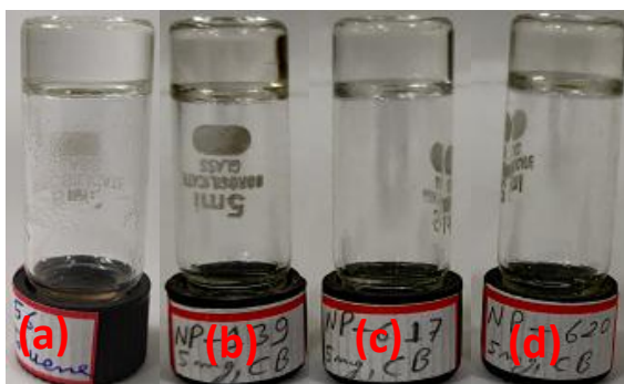
Figure S3. Gels from Chlorobenzene (a) 2b (0.2% w/v), (b) 2d (0.5% w/v), (c) 3'a (0.5% w/v), (d) 3'd (0.5% w/v).
