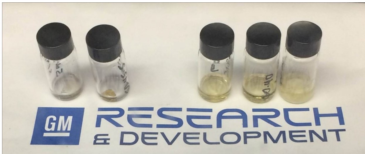
SFigure 2. The (\text{Li}_2\text{S})_{50}(\text{GeS}_2)_{45}(\text{GeO}_2)_5 glass (second from left) is also insoluble in glass in 1:1 (v/v) DME:DOL after two weeks just like the (\text{Li}_2\text{S})_{60}(\text{SiS}_2)_{28}(\text{P}_2\text{S}_5)_{12} glass (first from left). As expected, a variety of (\text{Li}_2\text{S})_x(\text{P}_2\text{S}_5)_{100-x} glasses (right group) are soluble in DME:DOL as evidenced by the solution's yellow color and turbidity.
