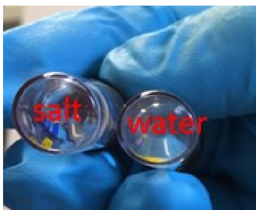
Figure S11: The gel after the overnight immersion in salt solution (0.1 M NaCl or 0.1 M CaCl 2 in water), as shown in the left vessel, stayed intact. In comparison, the gel after the overnight immersion in pure water, as shown in the right vessel, dissolved into pieces.
