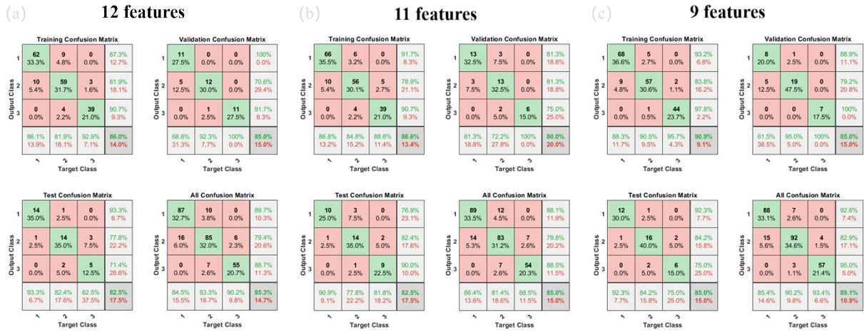
Fig. S11. Performance evaluation of the ANN algorithm. (a-c) The classification result in the training data set, validation data set, test data set and all data, using the ANN algorithm with 12 features, 11 features, and 9 features, respectively. Here, “1” represents BCC structure; “2” represents the BCC + FCC phase; “3” denotes the FCC phase.
