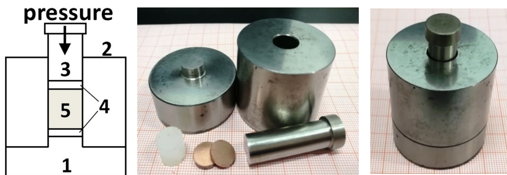
Fig. S4. The compression mould used for the V_S measurements. It contains: 1) a bottom, 2) a vessel, 3) a driving piston, 4) two copper gaskets, and 5) sample.
