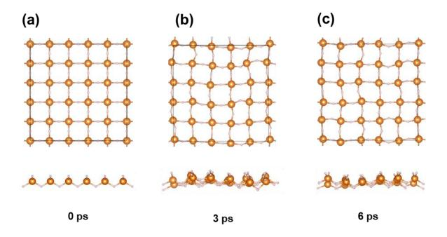
**Figure S2.** Snapshots (top and side views) of  $5 \times 5 \times 1$  supercell of 2D *P-4m2* MgH<sub>2</sub> at the (a) 0 ps (b) 3 ps and (c) 6 ps at 300K
