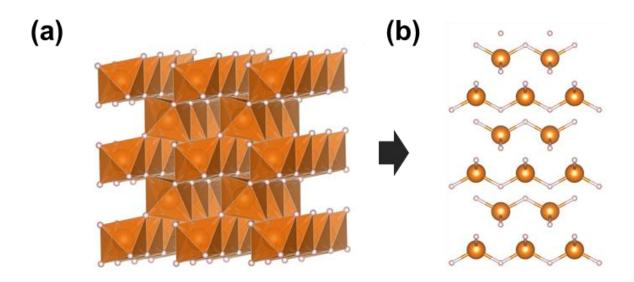
**Figure S1.** Two phases of MgH<sub>2</sub>, (a) the tetragonal MgH<sub>2</sub> with symmetry of  $P4_2/mnm$ ,  $\alpha$ -phase and (b) the layered bulk structure of 2D II-phase,  $P4_2/nmc$ .
