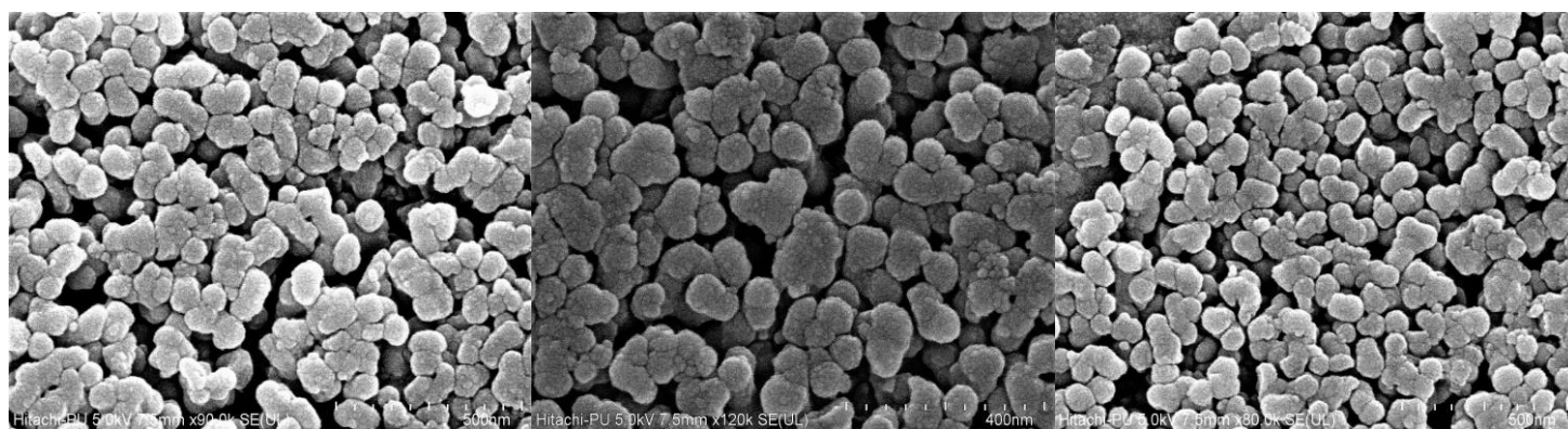
Fig S19. FESEM images of Fe 3 O 4 @SiO 2 @Silane at different magnifications
