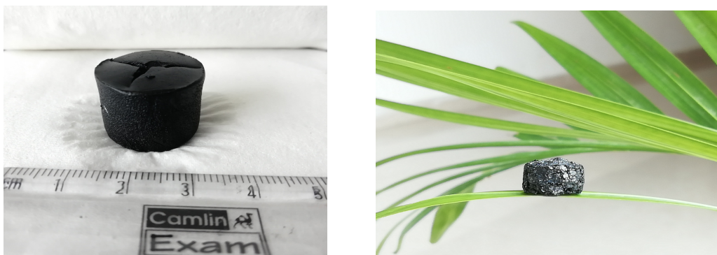
S1.2: pictures showing NS-rGO3 hydrogel , NS-rGO3 aerogel after freeze drying
