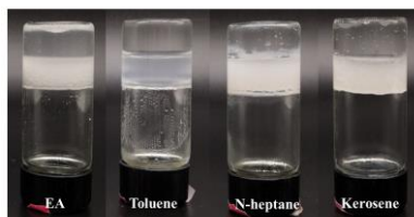
Fig. S3 Pictures of HSA-N phase-selectively gelate organic phase in an oil-water mixture.
