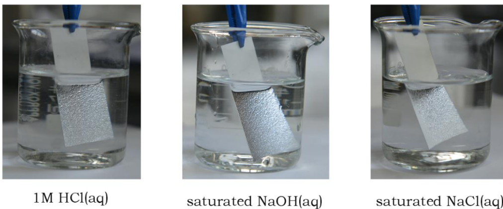
Fig. S5 Photographs the PU/DE@HD-POS coatings after soaked in various corrosive liquids for 1 h.
