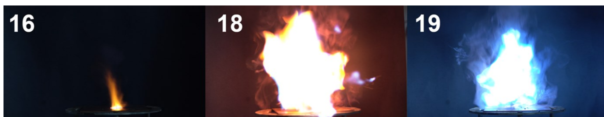
Fig. S30 Results of the hot plate tests of copper perchlorate compounds 16 , 18 , and 19 .
