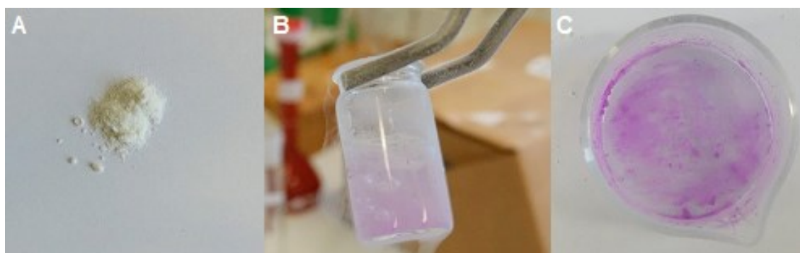
Fig. S31 [\text{Fe}(\text{C}_3\text{tz})_6](\text{ClO}_4)_2 ( 15 ) at room temperature (A) and cooled with liquid nitrogen (B, C) revealing a thermochromic effect.
