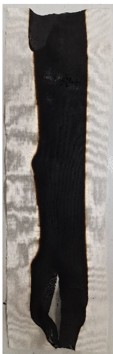
Fig. S3 Photos of treated cotton fabrics with 10% PBTCA after vertical flammability test
