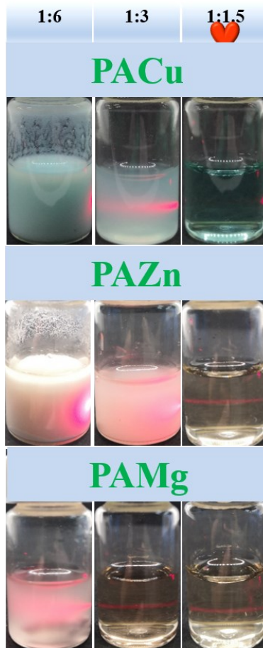
Figure S1. The solubility of divalent metal ion phytate in aqueous solution (0.1 g/mL) in different proportions.
