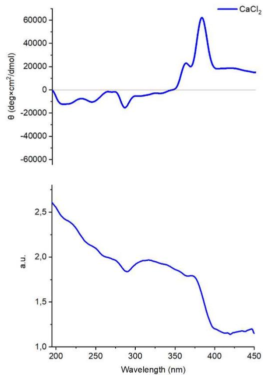
**S28:** CD spectrum of CaCl<sub>2</sub> gel and corresponding absorption spectrum
