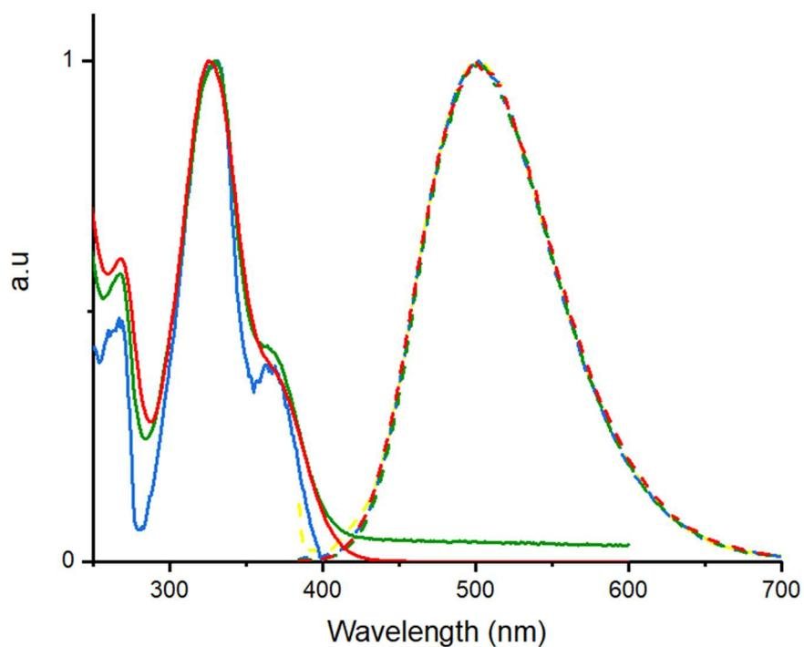
S15. Normalized absorption (solid line) and emission spectra (dashed line) of aqueous basic solutions of **1** at  $10^{-6}$  M (yellow),  $10^{-5}$  M (blue),  $10^{-4}$  M (green),  $10^{-3}$  M (red) concentration. The absorption at  $10^{-6}$  M concentration was too weak to be recorded in the same conditions.
