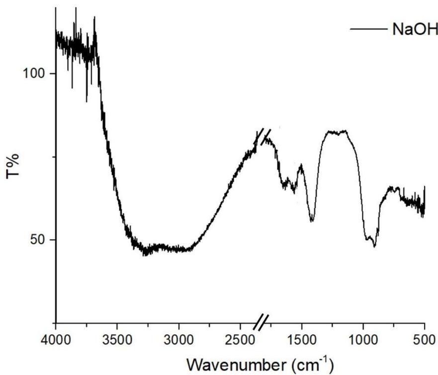
S21. ATR-FTIR spectrum of NaOH-gel.
