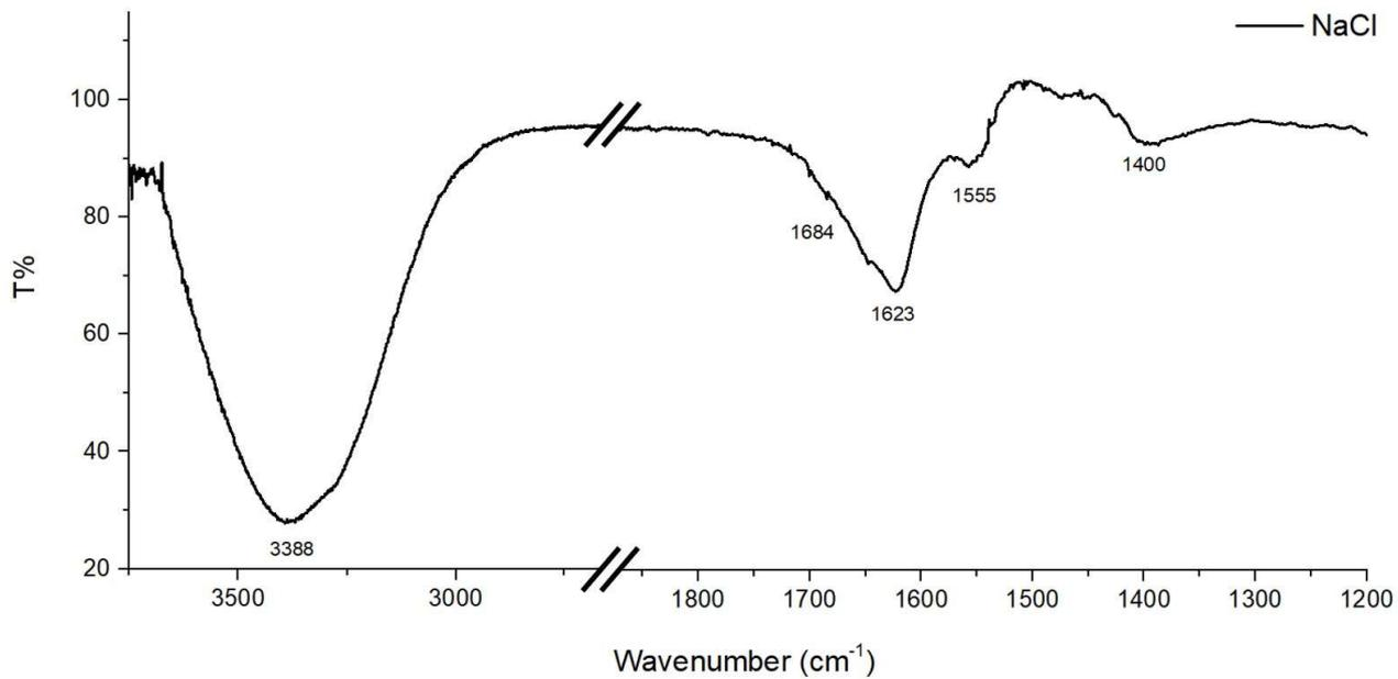
**S18.** ATR-FTIR spectrum of NaCl-gel.
