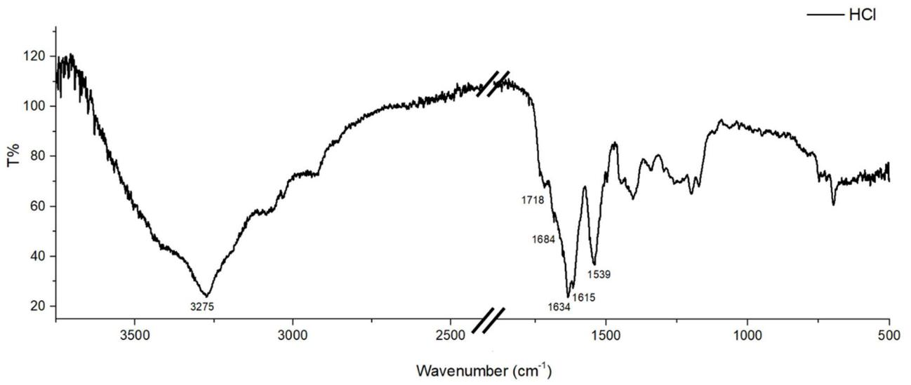
**S16.** ATR-FTIR spectrum of HCl-gel.
