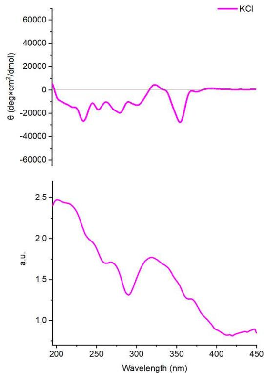
**S26:** CD spectrum of KCl gel and corresponding absorption spectrum.
