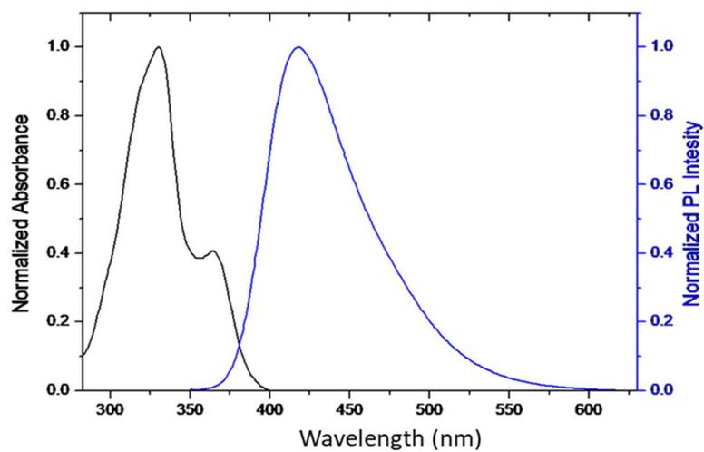
S3. Normalized absorption (black line) and emission (blue line) spectra of **2** in dichloroethane.
