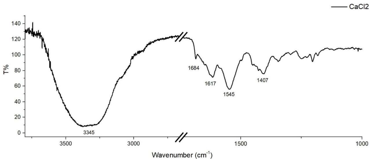
S20. ATR-FTIR spectrum of CaCl<sub>2</sub>-gel.
