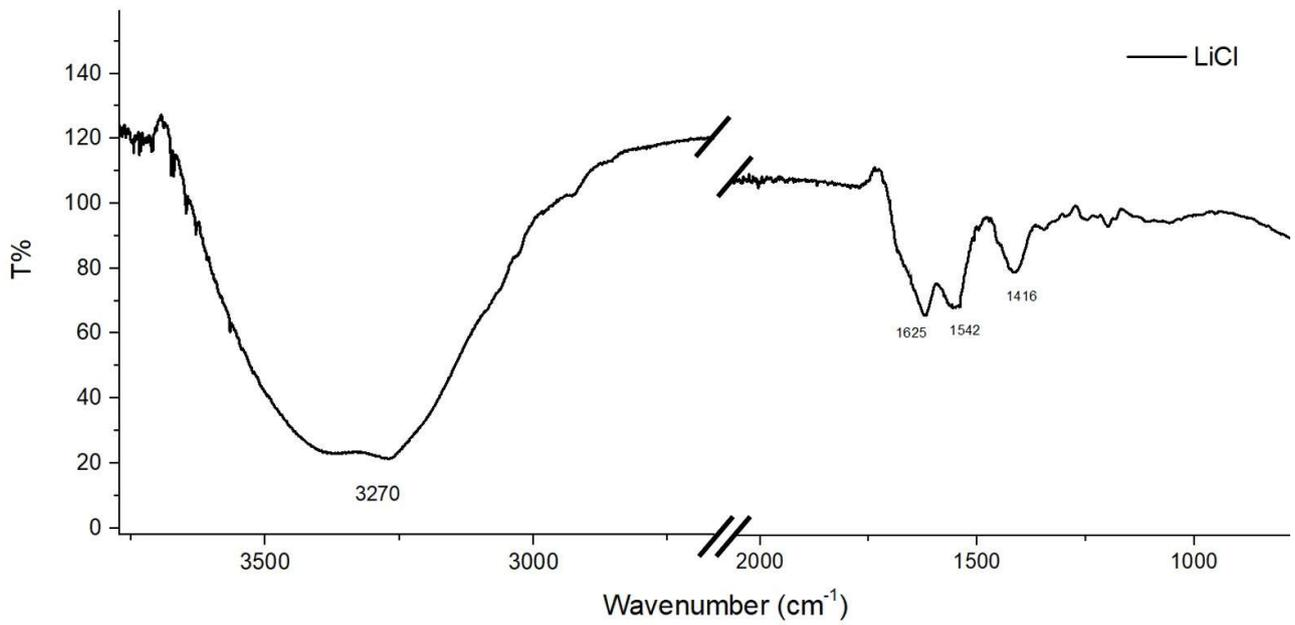
**S17.** ATR-FTIR spectrum of LiCl-gel.
