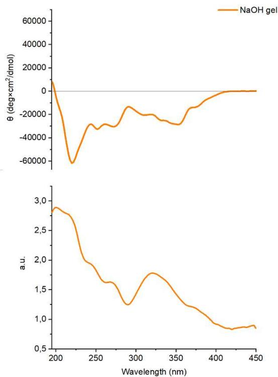
**S27:** CD spectrum of NaOH gel and corresponding absorption spectrum.
