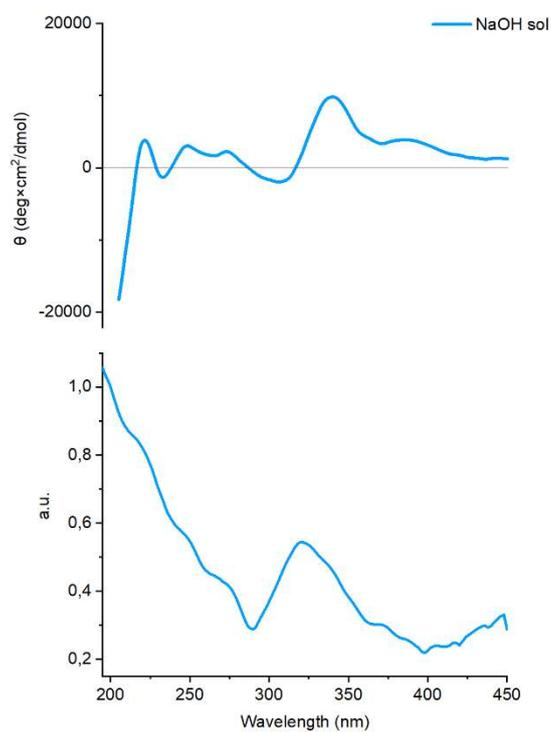
**S22:** CD spectrum of NaOH solution and corresponding absorption spectrum.
