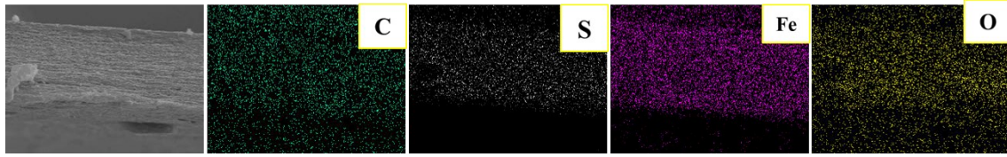
Figure S4. The cross section SEM and the corresponding elemental mapping images of rGO/CNTs/Fe 2 O 3 /PEDOT:PSS paper.
