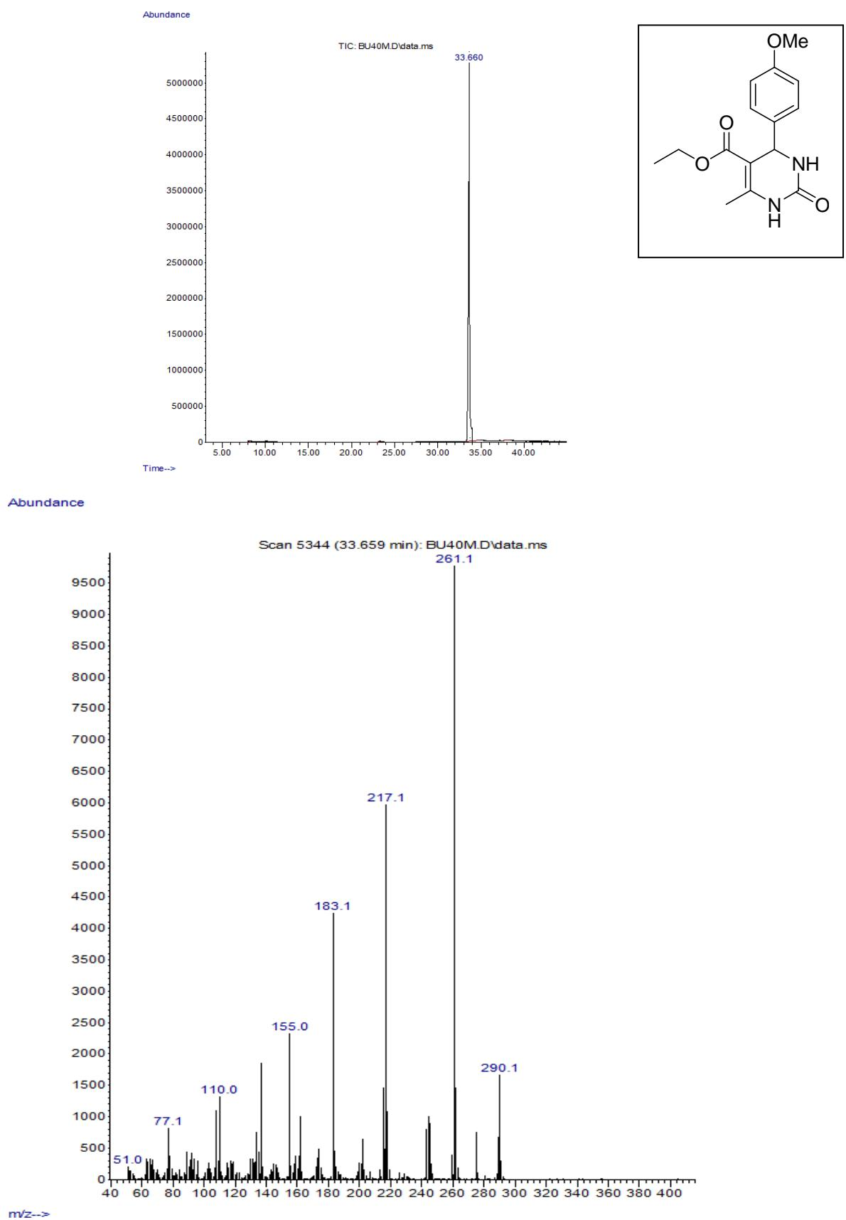
Gas chromatogram and mass spectrum of B5 (MW: 290)
