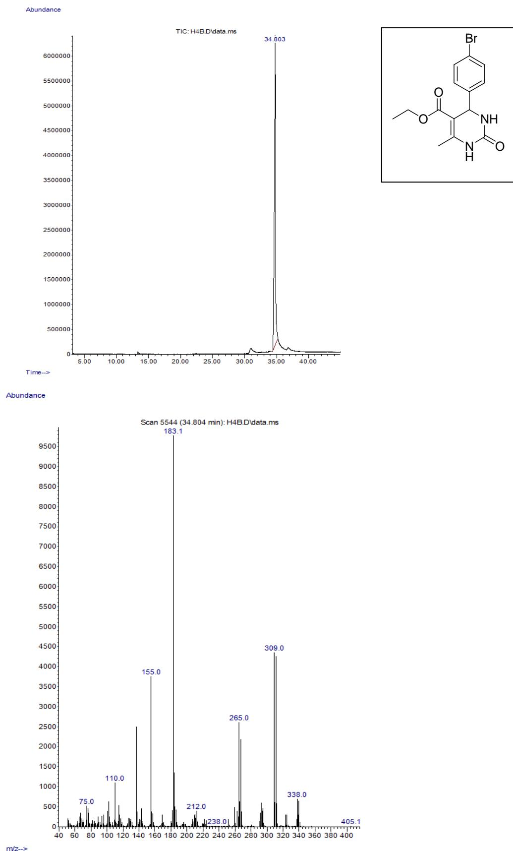
Gas chromatogram and mass spectrum of B4 (MW: 290)
