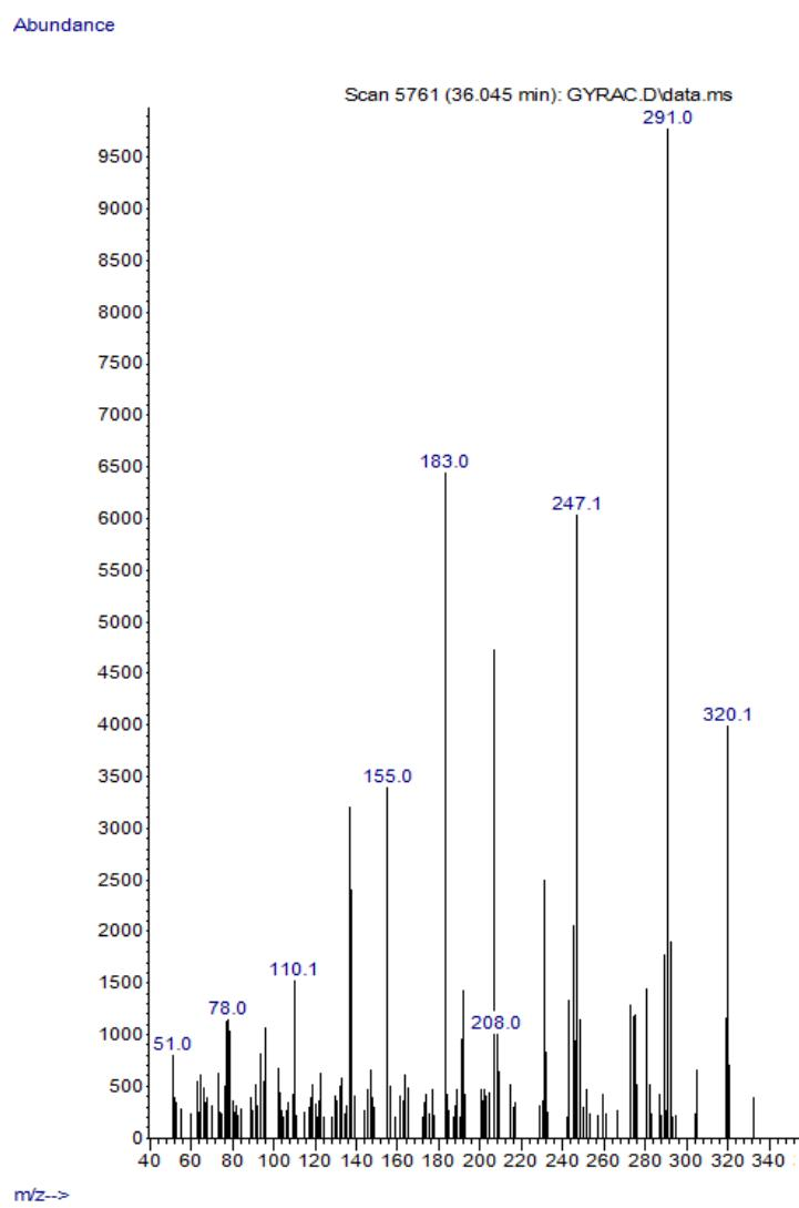
Gas chromatogram and mass spectrum of B7 (MW: 266)
