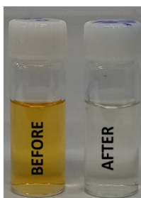
Figure S5. Image of MO dye before and after photocatalytic degradation using \text{TiO}_2@\text{Ag}@\text{LaFeO}_3 NRs under illumination of simulated light source.
