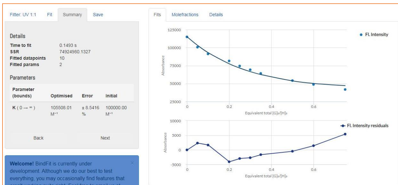
Fig. S16: Bindfit plots for Hg 2+ -binding by (a) 3 in 1:2 (non-cooperative) stoichiometry and (b) 4 in 1:1 stoichiometry from fluorescence titration using L-BFGS-B fit. Screenshots taken from the website supramolecular.org .
