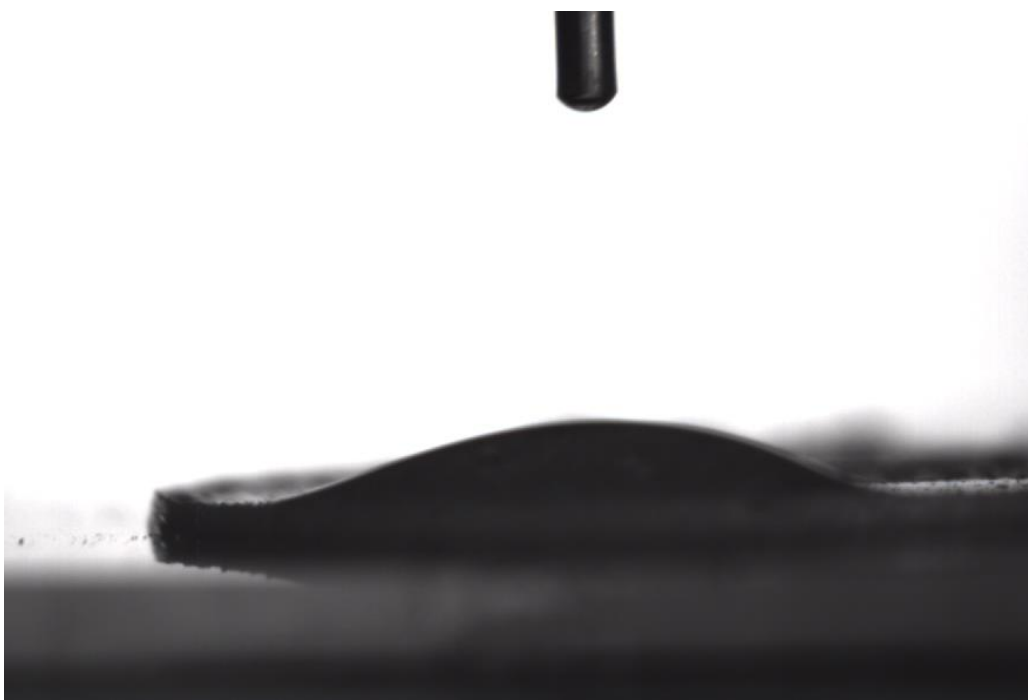
Fig. S5 The measurement of water contact angles for P(DVB-VIM).
