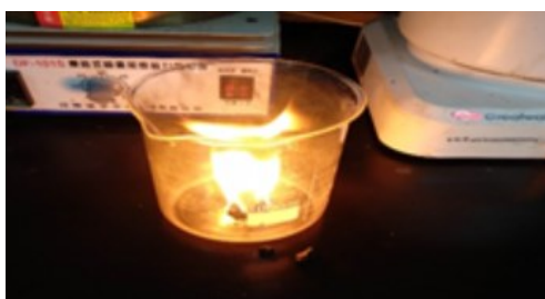
Figure S15. Pump oil absorption and combustion experiment
