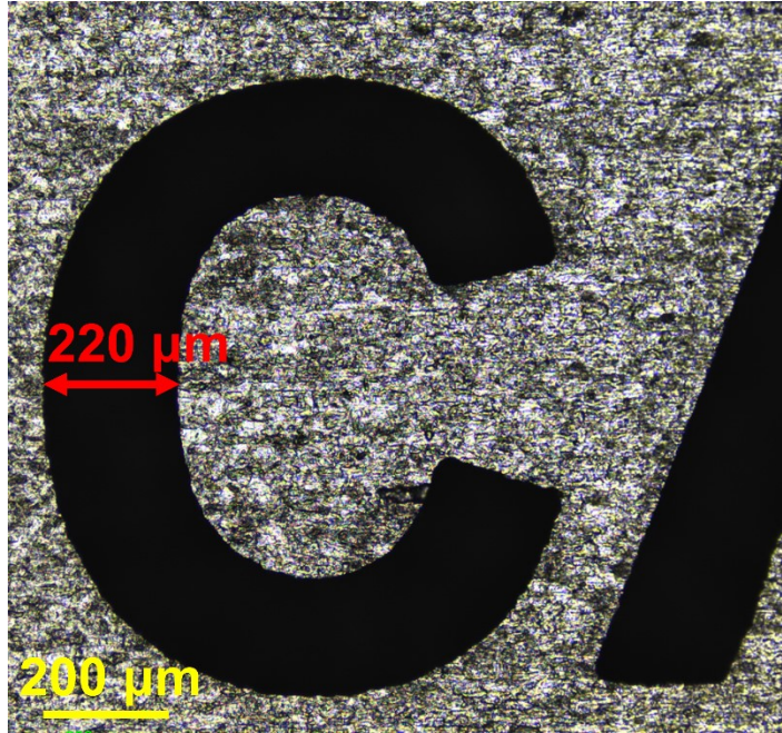
Figure S11. Optical microscope photograph showing the line width of the smallest CAEP letters in the mask.
