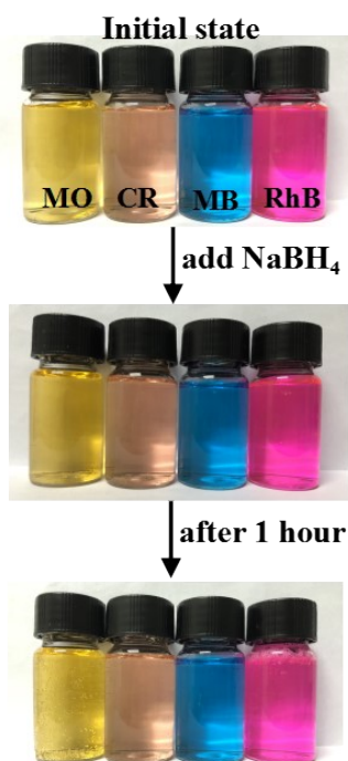
Figure S10 Photograph of dye molecules before and after addition of \text{NaBH}_4 without catalysts.
