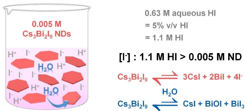
Figure S9. Schematic showing the plausible reason for the \text{Cs}_3\text{Bi}_2\text{I}_9 ND stability in 0.63 M saturated HI solution.
