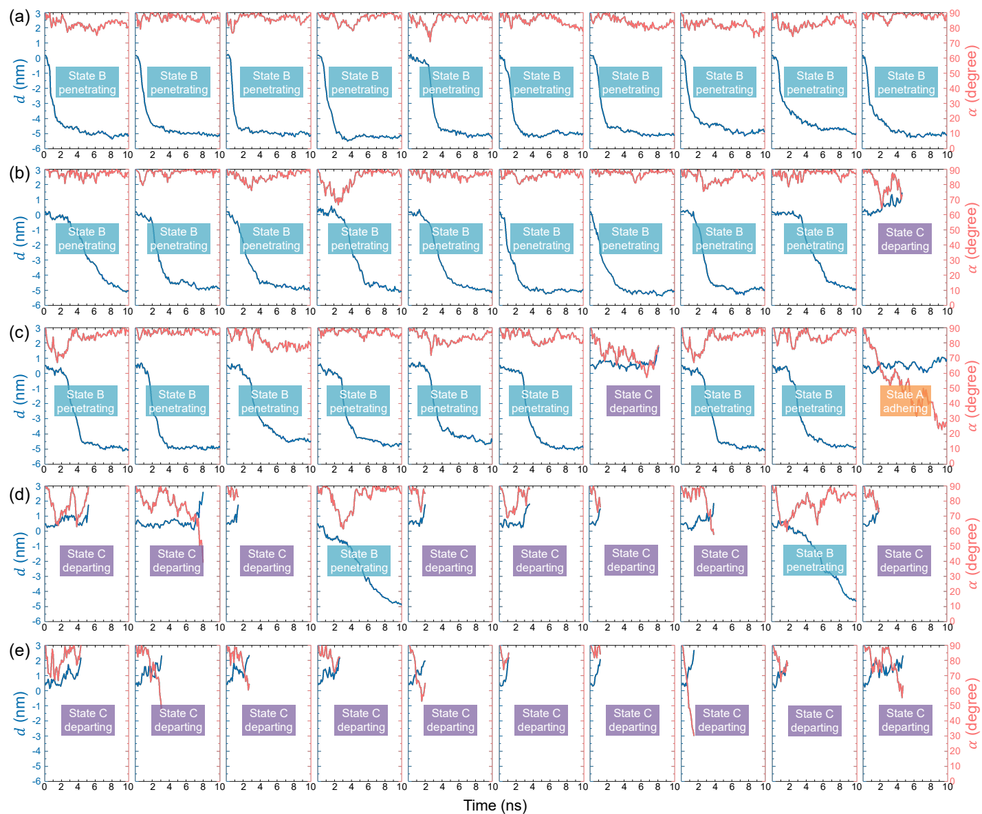
Fig. S10 Initiating from the orientation \vartheta = 45^\circ and \varphi = 90^\circ , temporal evolution of nanosheet position and orientation, as well as verdict of the final interaction state, when the graphene nanosheet interacts with C16:0-18:1 (a) PA, (b) PE, (c) PG, (d) PI, and (e) PS bilayer. 10 independent simulations were performed for each kind of phospholipid bilayer.
