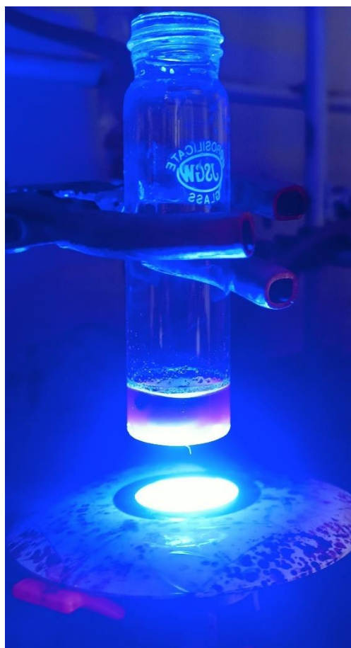
Figure FS1. Experimental set-up employed during photocatalytic reactions. Hyglow 3W blue LED (HY 124 - 3watt gemini E17 Blue) was used for the irradiation purpose.
