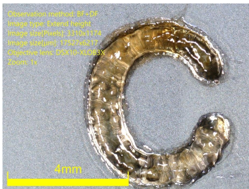
Photo S1. 3D hydrogel inscription made by the free-radical photopolymerization of mixture HEA/water (1/1 wt.) in the presence of a two-component photoinitiating system based on CA-CDs (0.2 wt. %) and IOD (2 wt. %).
