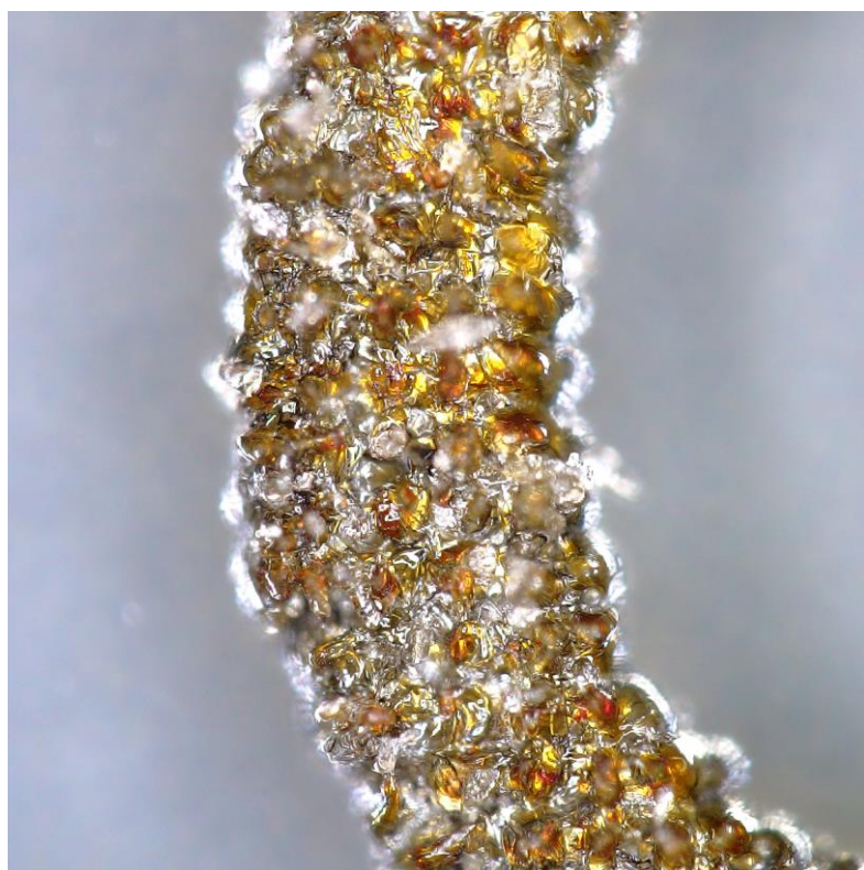
Photo S2. 3D inscription made by the cationic photopolymerization of vinyl monomer (TEGDVE) in the presence of a two-component photoinitiating system based on CA-CDs (0.2 wt. %) and IOD (2 wt. %).
