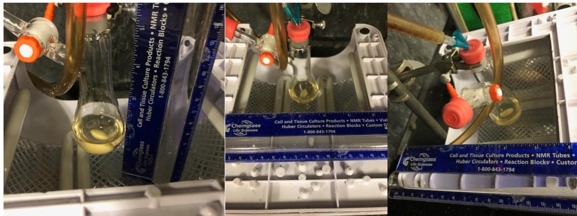
**Figure S14.** Schlenk flask set up in relation to UV source. UV source was equipped with four UV bulbs. Schlenk flask was positioned centrally and 1 cm from the bottom of the light source.
