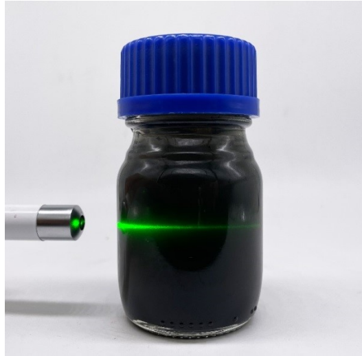
Fig. S4 The Tyndall phenomenon of the as-obtained \text{Ti}_3\text{C}_2\text{T}_x MXene suspension.
