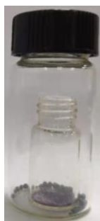
Fig. S11. The setup for iodine vapor adsorption.
