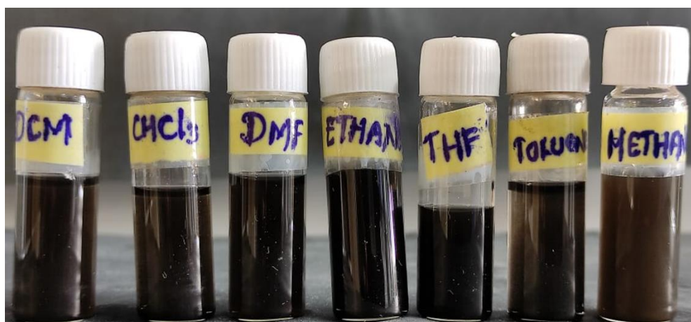
Figure S10: FG-DTC powder (5 mg) dispersed in 2 mL of polar, medium and non-polar solvents
