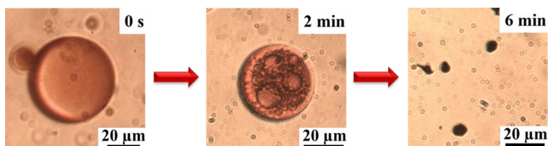
Fig. S6 OM images demonstrating the spontaneous permeation of aqueous phase into the emulsion droplets and the deformation of emulsion droplets with the evaporation of chloroform. The initial stage ( i.e. , 0 min) shows that the initial homogeneous emulsion droplets are spherical. With the volatilization of chloroform, the homogeneous spherical emulsion droplets are gradually permeated by surfactant aqueous solution ( i.e. , 2 min). Eventually, the spherical emulsion droplets spontaneously break up into flat droplets due to the excessive penetration of the external aqueous solution ( i.e. , 6 min).
