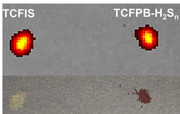
Figure S10. Fluorescence imaging for powder of TCFIS and TCFPB-H 2 S n under IVIS. Fluorescent emission was collected from 600 to 840 nm. \lambda_{\text{ex}} = 570 nm.
