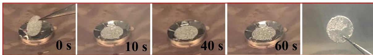
Figure S2 Time evolution images of thermal infusion molten Li process into bare Ni foam (conducted at a heating platform, 300 °C).
