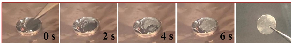
Figure S3 Time evolution images of thermal infusion molten Li process into Au/NNS-NF (conducted at a heating platform, 300 °C).
