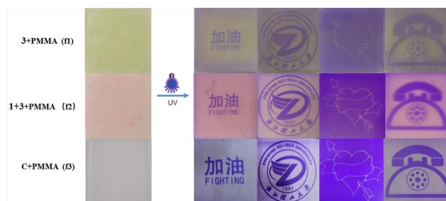
Figure S16 Images obtained after UV light on PMMA film (f1, f2, f3).
