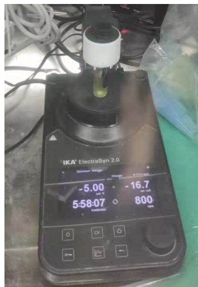
Current controlled electrolysis ( ElectroSyn 2.0 apparatus, IKA)
