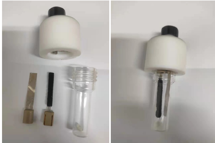
Reticulated Vitreous Carbon (RVC, Right) and Pt(Left)
