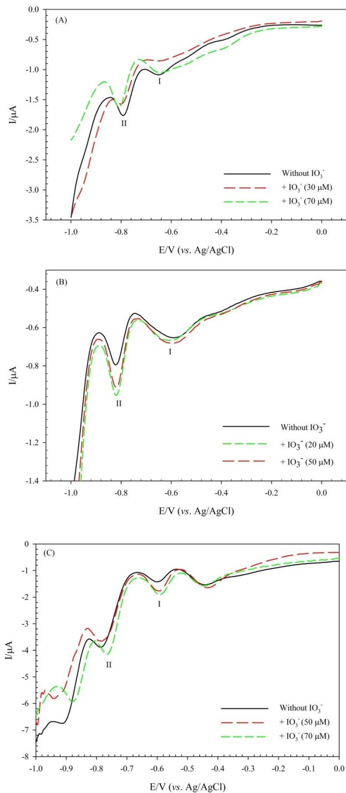
**Figure S3** SWV responses for the determination of  $\text{IO}_3^-$  in (A) mineral water, (B) tap water, and (C) commercial edible iodized salt prepared in the  $\text{HClO}_4$  solution (0.1 mol  $\text{L}^{-1}$ , pH=1.5) at (bdpy)SiW<sub>11</sub>Ni/P-ERGO/GCE); scan rate 50  $\text{mVs}^{-1}$ .
