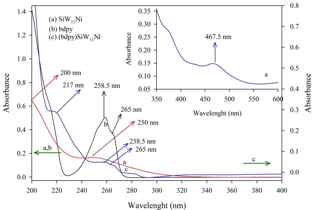
**Figure S2** UV-Vis spectra of  $\text{SiW}_{11}\text{Ni}$  (a),  $\text{bdp}$  (b) in deionized water, and  $(\text{bdp})\text{SiW}_{11}\text{Ni}$  (c) in acetonitrile. The inset shows the UV-Vis spectrum of  $\text{SiW}_{11}\text{Ni}$  in deionized water at 350-600 nm.
