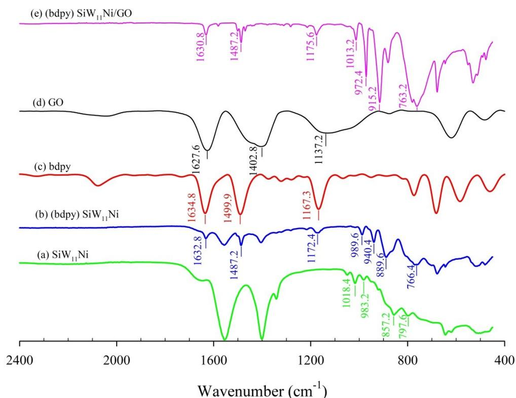
**Figure S1** ATR-FTIR spectra of SiW<sub>11</sub>Ni (a), (bdpy)SiW<sub>11</sub>Ni (b), bdpy (c), GO (d), and (bdpy)SiW<sub>11</sub>Ni/GO (e)
