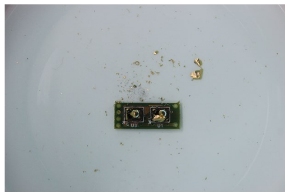
Fig. S7. Photo images of non-coating circuit board immersed in 30 vol% nitric acid solution. Fragmented copper alloy spread into the solution after 3 hours (a) and continued after 5 hours (b).
