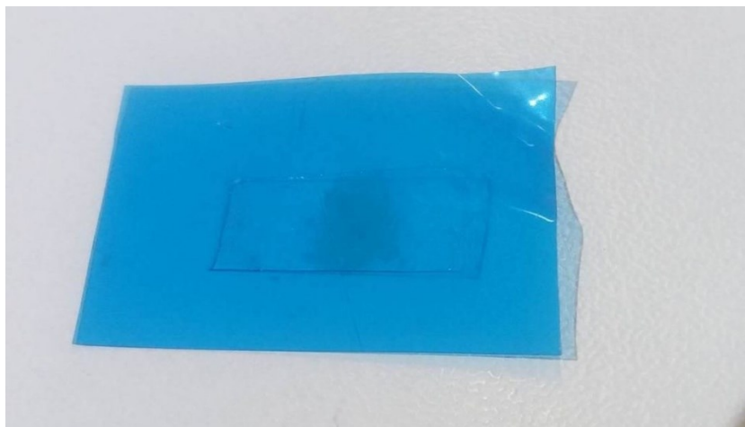
Figure S7. Dry transfer from the PDMS after EBL to the PET substrate.
