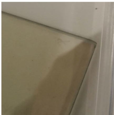
Figure S1. Photograph of the MoS 2 film grown on 10x10 cm glass substrate.
