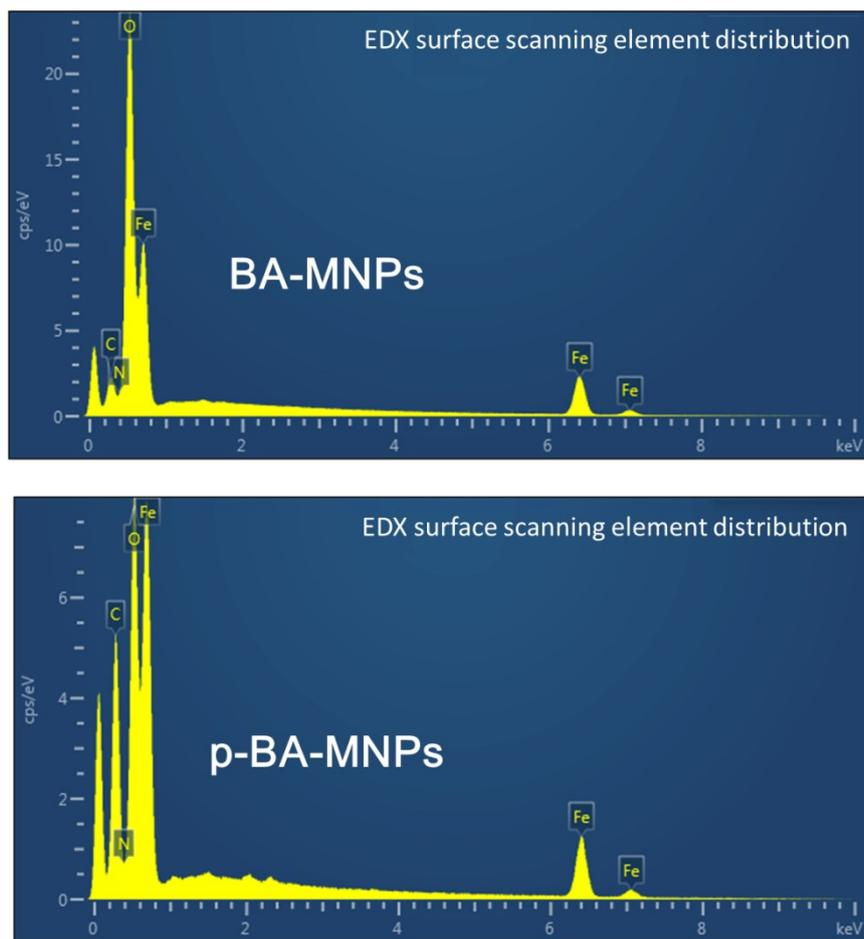
**Fig. S1.** Energy dispersive spectroscopy (EDS) of BA-MNPs and p-BA-MNPs.
