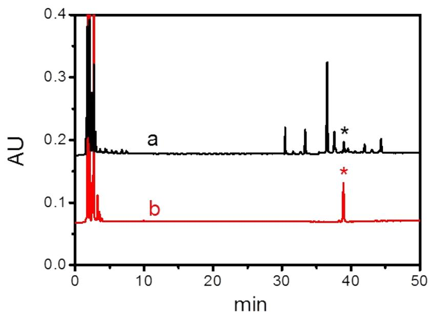
**Fig. S6.** Chromatograms of ginsenoside Re spiked (100 ng/mL) human serum, (a) direct analysis and (b) after enrichment with Apt Re-3@MNPs. \* indicates ginsenoside Re.
