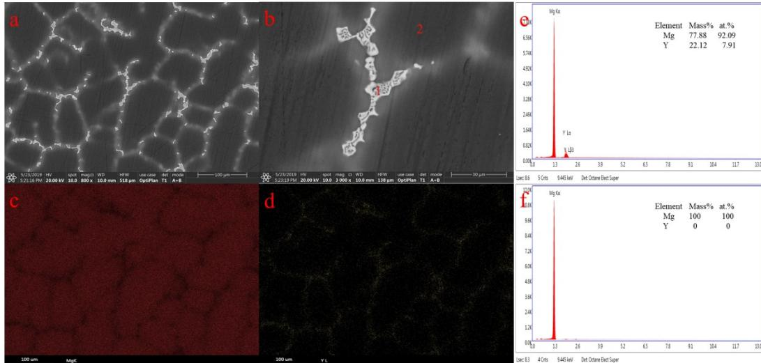
SEM (a, b), EDS mapping (c, d) and quantitative (e, f) analysis of Mg-Li-Y alloy obtained by galvanostatic electrolysis (-0.4 A) in LiCl-KCl-MgCl<sub>2</sub> (8 wt. %)-YCl<sub>3</sub> (2 wt. %) melts on the W electrode ( $S=0.322\text{ cm}^2$ ) at 973 K.
